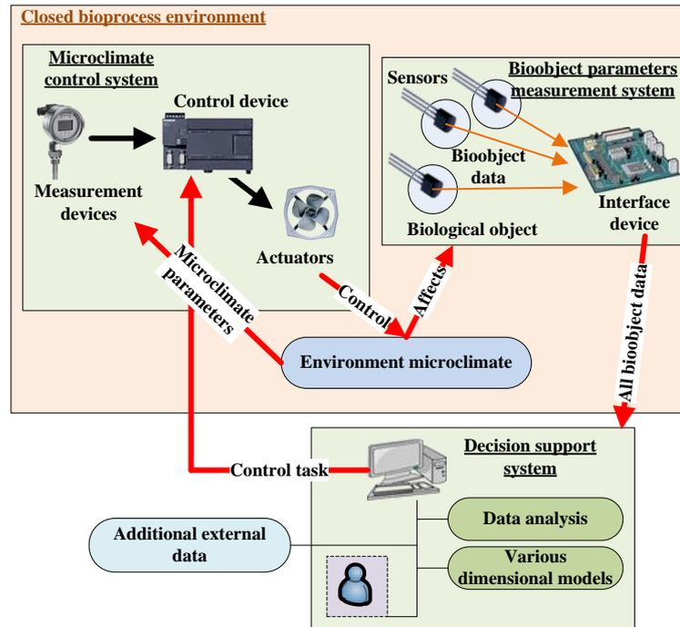
**Fig. 1.** Architecture of computer control system (Zacepins, 2013)
