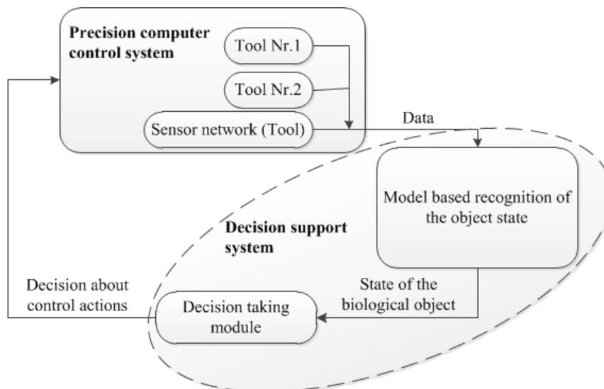
**Fig. 2.** Diagram of information flow for DSS implementation in PCC
