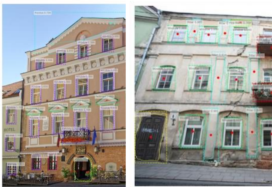
Fig. 7. The results of AI training: highlighted are different classes of objects identified by AI engine on photos taken at different angles towards the facade of a building
