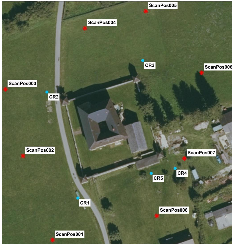
Figure 2: The figure clearly shows the selected scanner positions (ScanPos###) and the locations of the drum reflectors (CR#) which were chosen in such a way that an optimal merging of the individual point clouds could be ensured. Note the group of trees on the right (eastern) edge of the image, which complicates the measurement and noticeably reduces the quality of the overall model.
