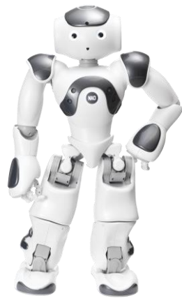
Figure 2. Humanoid robot NAO V6 that was used in developing HRI in Lithuanian language
