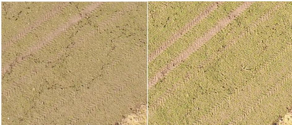
Figure 1. Example with combination of two images from neighbour fields that can't be stitched together (images taken from height of 45 meters)
