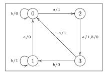
Fig. 7. Transition diagram of *Mealy machine*  $M_{me1}$
