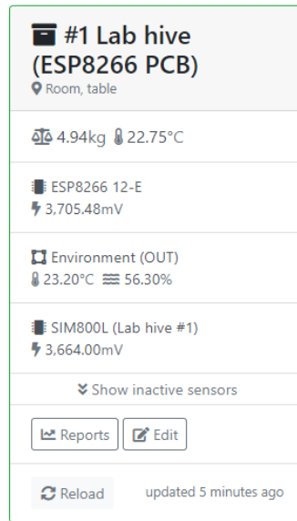
Fig. 5. SAMS data warehouse Dashboard colony card with sensor data
