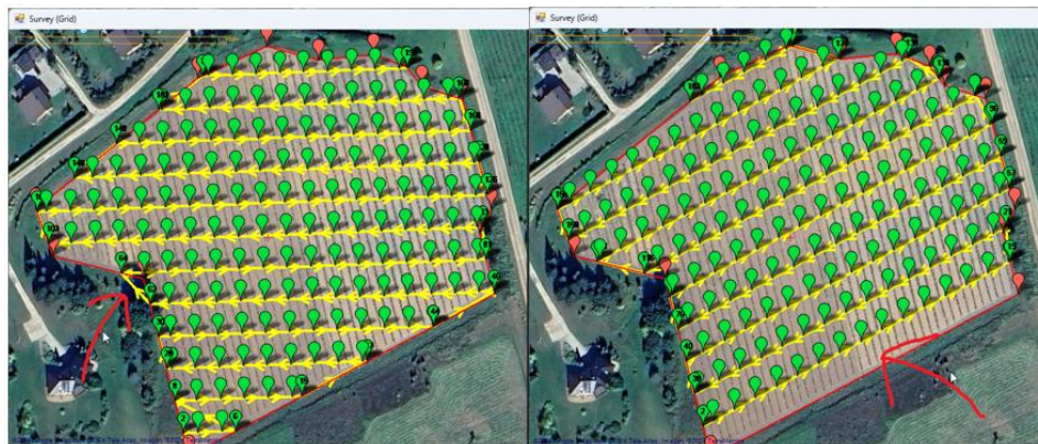
Figure 2. Routes where a drone could fly into a tree (image links) or not the entire area covered (image right)
